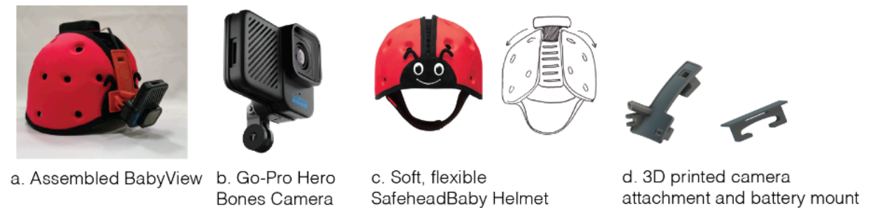
Figure 2. Overview of the BabyView Camera design process, showing (a) the assembled device, (b) the original camera, (c) babysafe helmet, and (d) and 3D printed mounting equipment.
