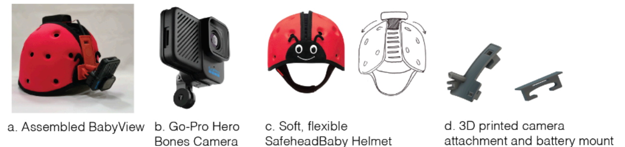
Figure 2. Overview of the BabyView Camera design process, showing (a) the assembled device, (b) the original camera, (c) babysafe helmet, and (d) 3D printed mounting equipment.
